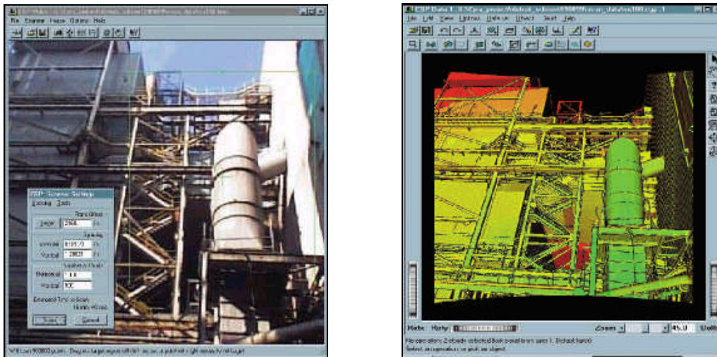
Figure 3.2 Source object and scan image from a Time-of-Flight scanner.
